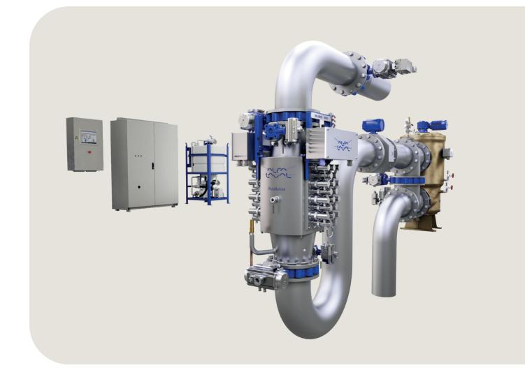
Alfa Laval's own ballast water management solution, Alfa Laval PureBallast, employs filtration and UV treatment. For all UV systems, there are two situations in which CWQ conditions could arise. The first is water with low UV transmittance, which could result in UV intensity below the SDL. The second is high sediment load, which could lead to increased differential pressure and cause filter clogging.
