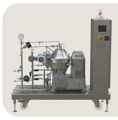
1935/2004. The metallic product contact parts are made of high-grade stainless-steel ensuring corrosion resistance and the non-metallic product contact parts, including gaskets and seals, are made of materials according to FDA requirement.
