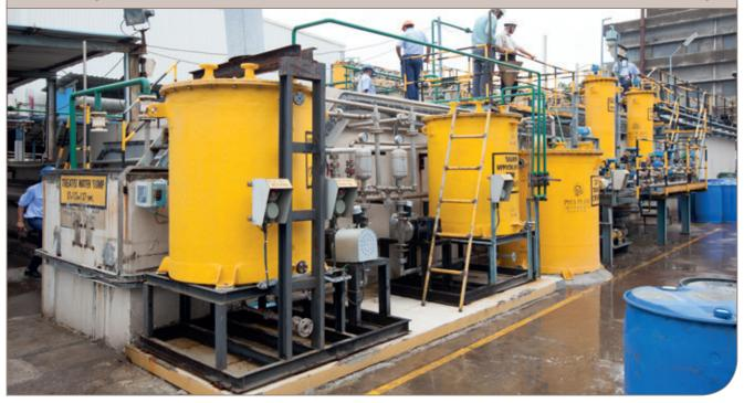
After side-by-side testing, speciality chemicals producer Galaxy Surfactants, India, chose Alfa Laval hollow sheet membrane bioreactors (MBRs) instead of flat sheet solutions for three industrial wastewater treatment plants. With MBR Galaxy will, after installation of reverse osmosis, be able to reuse the water for domestic purposes, successfully pursuing their zero liquid discharge (ZLD) strategy and saving fresh water resources.
