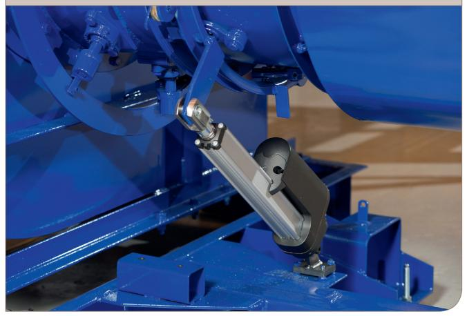
The electric FD (forced-draught) fan actuator upgrade kit contains everything needed to replace the original pneumatically operated fan actuator of your Alfa Laval Aalborg burner with an electrically operated actuator. This results in a highly accurate and maintenance-free damper positioning system.
